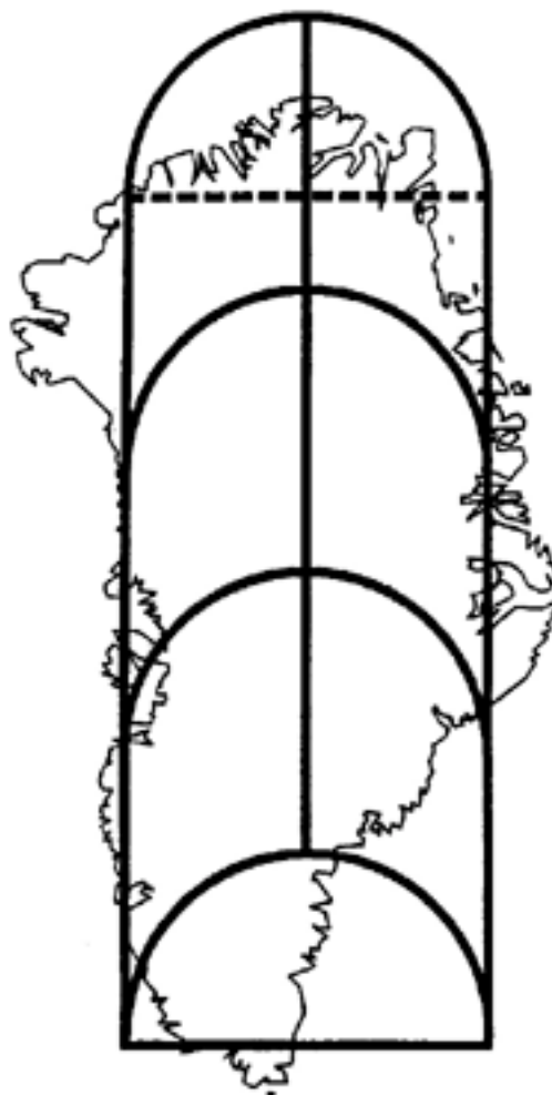
Figure 10. Schematic of bindschadler (1985) model. Extrapolating the 2-D model to three dimensions by a scaling factor of 5000 km is equivalent to assuming two parabolic cylinders back-to-back, with transverse (longitudinal) length of 2500 cm. Greenland is drawn to the same scale.
